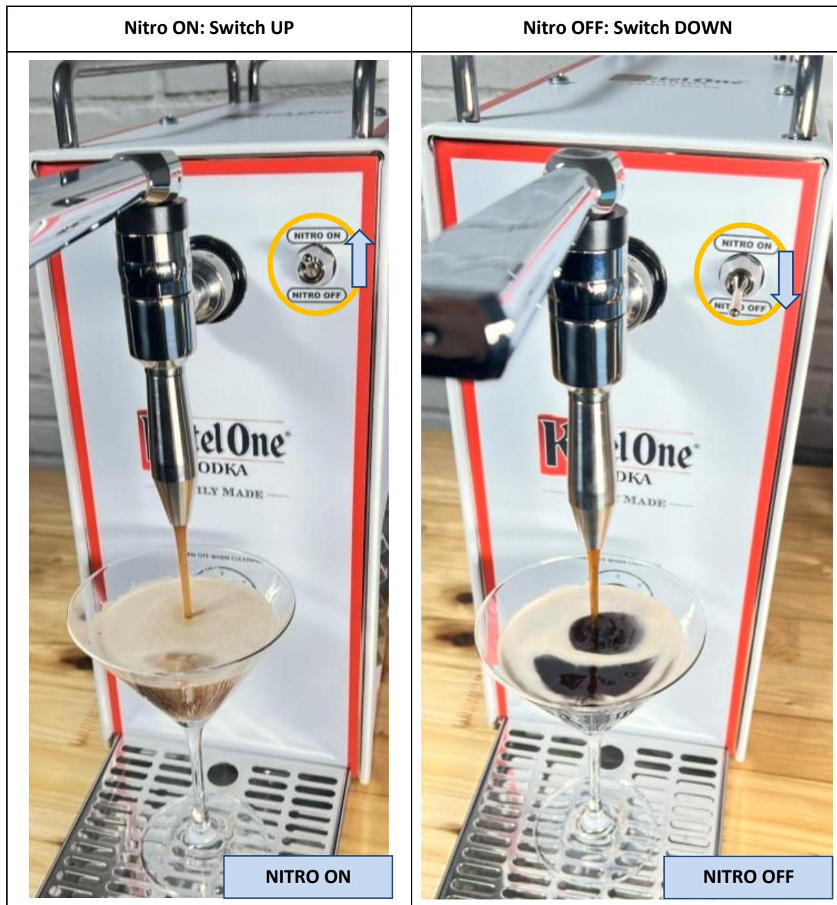
When changing from NITRO-ON to NITRO-OFF it takes about 50 ml of product until the remaining nitro gas is out. Open & close the tap handle a couple of times (3-4) and dispense the 50 ml in small batches, like this the gas in the tap is flushed out faster.
