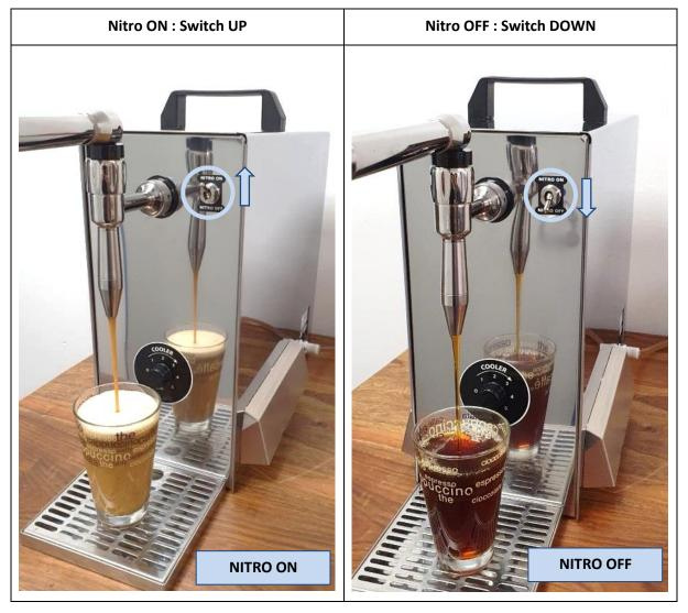
When changing from NITRO-ON to NITRO–OFF it takes about 50 ml of coffee until the remaining nitro gas is out. Open & close the tap handle a couple of times (3-4) and dispense the 50 ml in small batches, like this the gas in the tap is flushed out faster.
