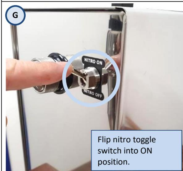
Flip nitro toggle switch into ON position.
