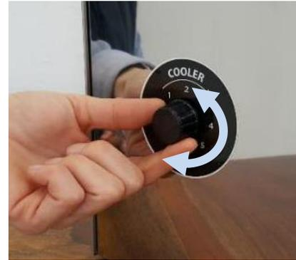
Dispensers used for coffee-cocktails can be set colder at customer's request. The temperature level is lowered by 6°C. The temperature of stage 7 is then: -1°C and the temperature of stage 1: 11°C. When tapping non-alcoholic beverages during cleaning and rinsing, the unit must be set to level 4 or lower (3,2,1) - otherwise the beverage may freeze. Level 4 corresponds to approx. 5°C.
