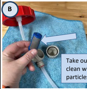
B Take out filter element and clean with water in case of particles or clogging.
