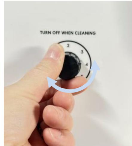
**When tapping non-alcoholic beverages during cleaning and rinsing, the unit must be set to level 4 or lower (3,2,1) - otherwise the beverage may freeze. Level 4 corresponds to approx.  $41^{\circ}\text{F}$ .**
