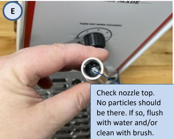
Check nozzle top. No particles should be there. If so, flush with water and/or clean with brush.
