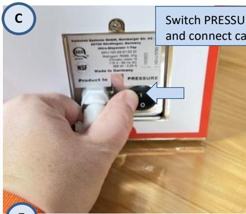
Switch PRESSURE ON and connect canister
