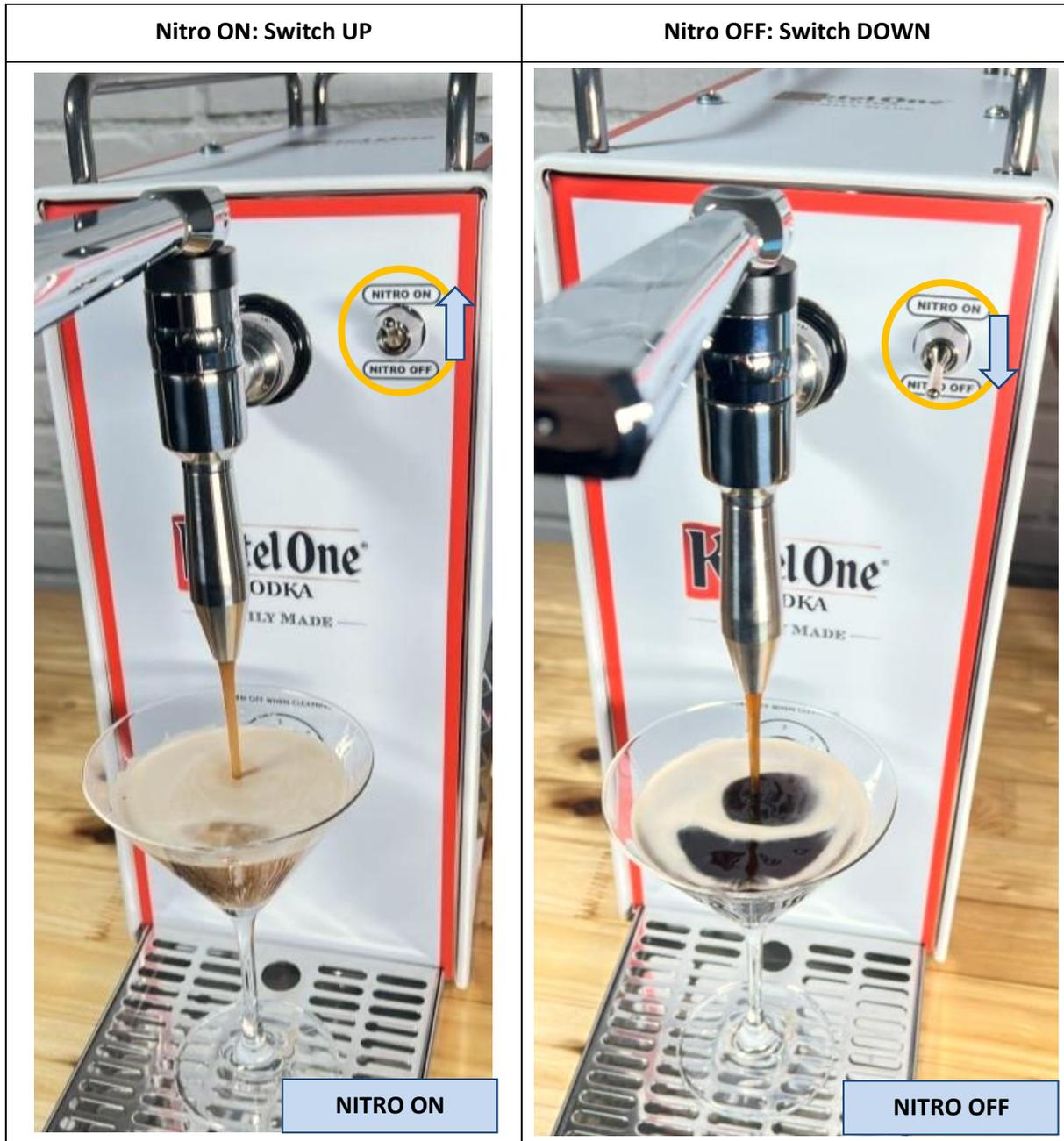
When changing from NITRO-ON to NITRO-OFF it takes about 50 ml (1.7 oz) of product until the remaining nitro gas is out. Open & close the tap handle a couple of times (3-4) and dispense the 50 ml (1.7 oz) in small batches, like this the gas in the tap is flushed out faster.
