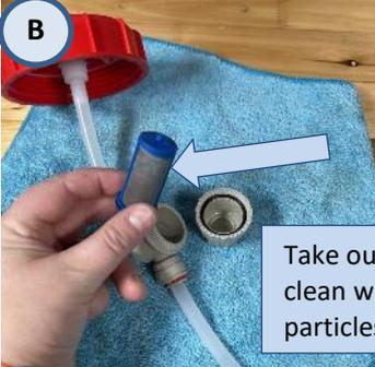
Take out filter element and clean with water in case of particles or clogging.
