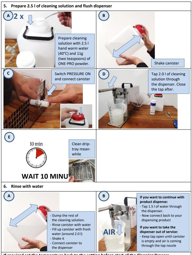
If required set the temperature back to the setting before start of the Cleaning Process
